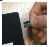
If you are using a Micro SD card which is over 32GB you will have to format the card to FAT32 first before it works.
