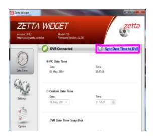
When the software is open and the device is connected, you should be able to see this Window above. Please select 'Sync Date Time to DVR' (Highlighted in the pink box above). This will set the device's time and date stamp to the Computer's time/date stamp.
