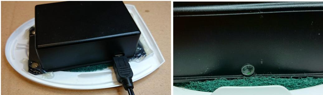
When the USB is inserted you should see a **green & orange light** showing through the window of the box to indicate that the device is taking charge (as shown in the above picture). For maximum power we suggest leaving the device on an overnight charge (**6 - 7 hours**).
