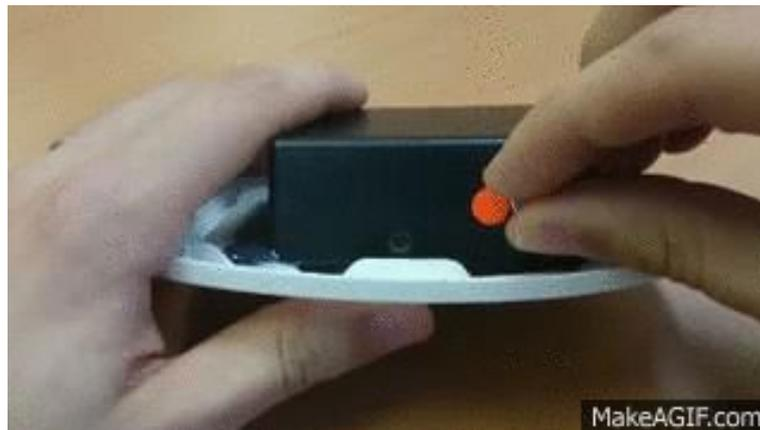
The device is now in recording mode and will record whenever it sees motion. Once you have finished recording simply hold the magnet to the device again and the light will glow **both green & orange** before going out, at this point the unit has switched off. We have made a short YouTube video so that you can see the power switch being used <http://goo.gl/KrPEO0>
