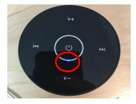
Hold your finger against the middle power button and hold it until the device starts to blink with blue lights, release your finger and replace it again and hold for about 10 seconds, the blinking lights should stop and an orange LED light should appear, followed by a solid red LED light- this means your device is recording.
